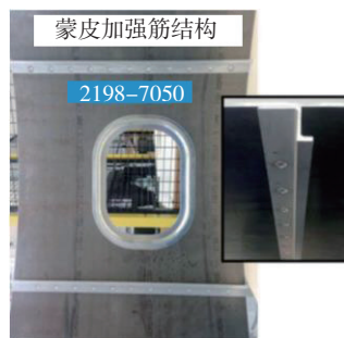
图20 飞机蒙皮和加强筋结构试验件 Fig.20 Sample for airplane skin and stiffener structure samples
