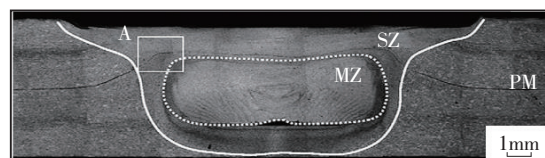
图17 典型回填式搅拌摩擦点焊接头分区 Fig.17 Different zones of refilled FSSW joint
